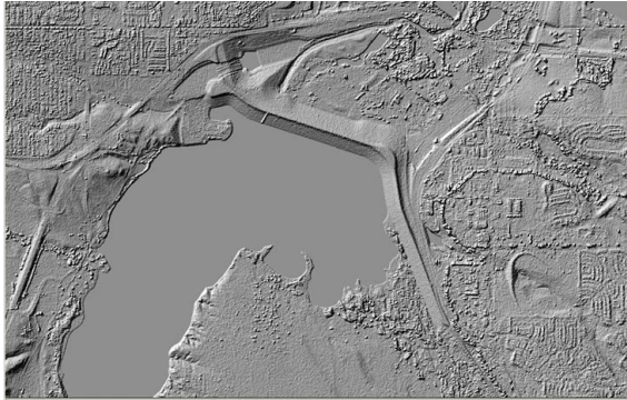
Figure 20. IFSAR collects the top reflective surface used to produce a digital surface model (DSM)
