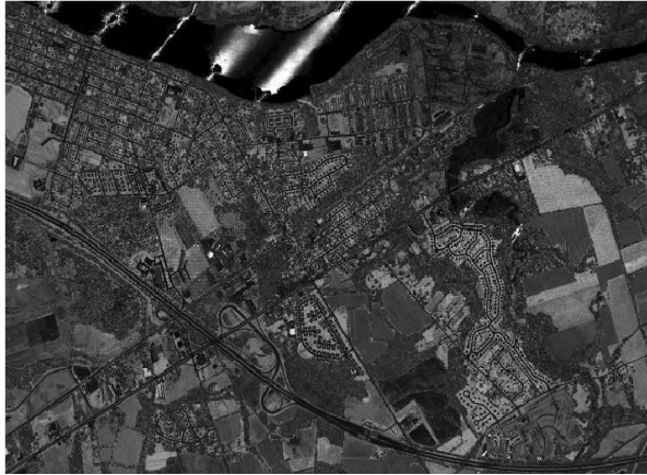
Figure 29. Intensity image showing streaks over water from multiple flight lines. This is not a problem because LiDAR measurements on water are already assumed to be unreliable and are classified separately as LAS Class 9. This entire image is usable for lidargrammetry.
