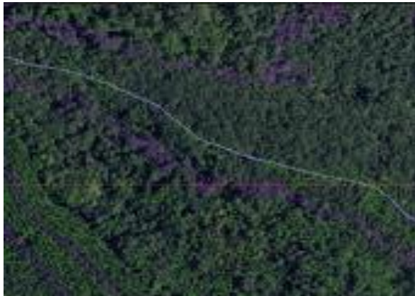
Figure 27. In spite of dense vegetation shown on this orthophoto in Florida, LiDAR data collected at a point density of 4 points/m 2 was still able to establish a hydro flow line for the dry drainage feature beneath.
