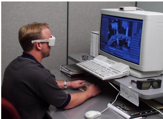
Figure 18. With manual photogrammetry, the compiler uses polarized glasses to see the left image with the left eye and the right image with the right eye, manually compiling spot heights where the bare earth terrain is visible in stereo and/or compiling 3D breaklines. Manually compiled contours are considered too expensive and time-consuming.
