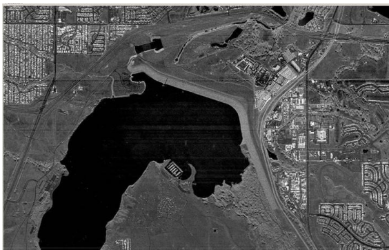
Figure 22. IFSAR ortho-rectified radar image (ORI) used to generate water masks, eliminating need for breaklines
